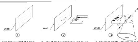
Speaker weight of 1.6Kg, must be chosen sSolid body by force, to avoid unstable speakers falling or injuries.
